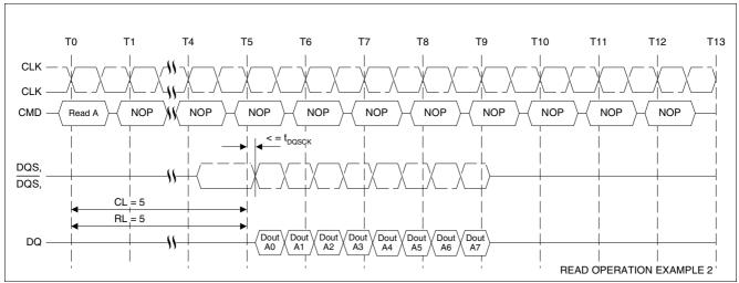
Figure 21 Read Operation Example 2: RL = 5 (AL = 0, CL = 5, BL = 8)
