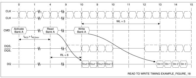
Figure 18 Read to Write Timing Example: Read followed by a write to the same bank, Activate to Read delay >  $t_{\text{RCDmin}}$ : AL = 1, CL = 5, RL = 6, WL = 5, BL = 4
