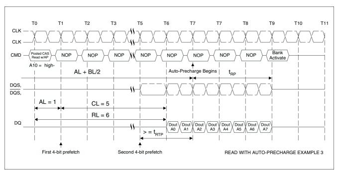
Figure 43 Read with Auto-Precharge Example 3, followed by an Activation to the Same Bank: RL = 6 (AL = 1, CL = 5), BL = 8,  $t_{RTP} \le 2$  clocks
