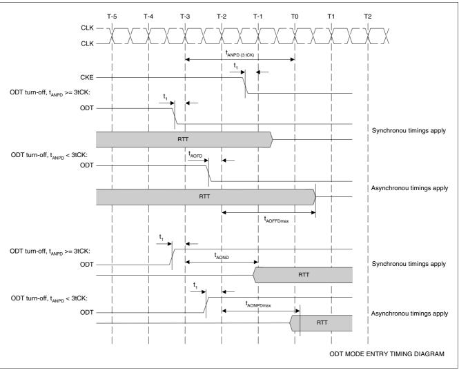
Figure 11 ODT Mode entry Timing Diagram
