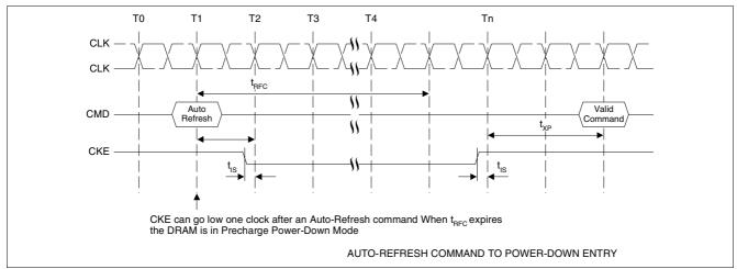
Figure 53 Auto-Refresh command to Power-Down entry
