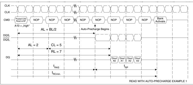
Figure 41 Read with Auto-Precharge Example 1, followed by an Activation to the Same Bank ( $t_{RC}$  Limit): RL = 7 (AL = 2, CL = 5), BL = 4,  $t_{RTP} \le 2$  clocks
