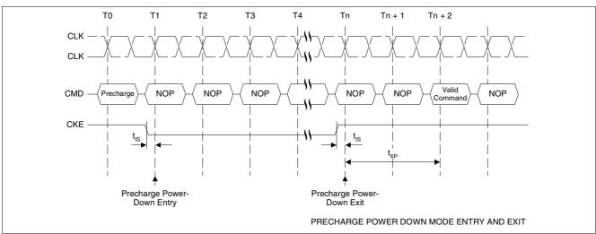
Figure 52 Precharge Power Down Mode Entry and Exit
