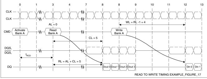
Figure 17 Read to Write Timing Example: Read followed by a write to the same bank, Activate to Read delay = *t*<sub>RCDmin</sub>: AL = 0, CL = 5, RL = (AL + CL) = 5, WL = (RL -1) = 4, BL = 4
