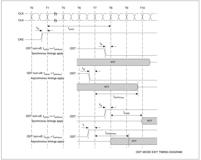
Figure 12 ODT Mode exit Timing Diagram
