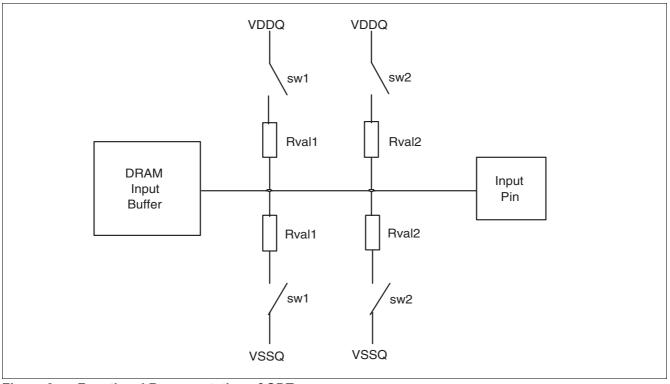
Figure 8 Functional Representation of ODT
