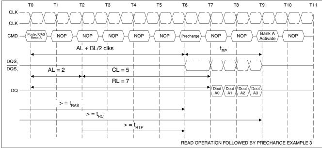
Figure 37 Read Operation Followed by Precharge Example 3: RL = 7 (AL = 2, CL = 5), BL = 4,  $t_{RTP} \le 2$  clocks
