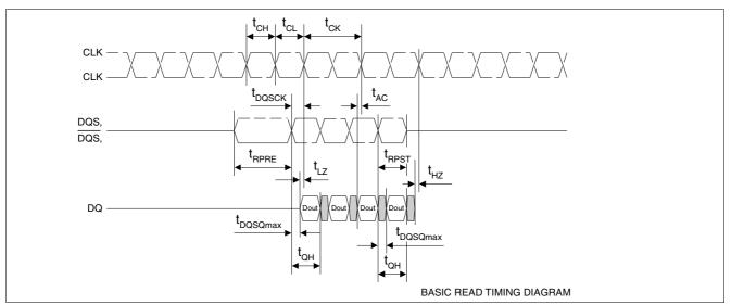
Figure 19 Basic Read Timing Diagram
