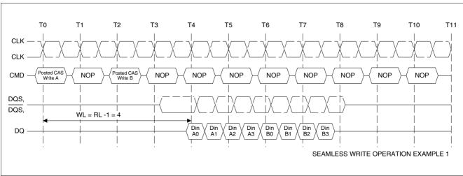
Figure 29 Seamless Write Operation Example 1: RL = 5, WL = 4, BL = 4
