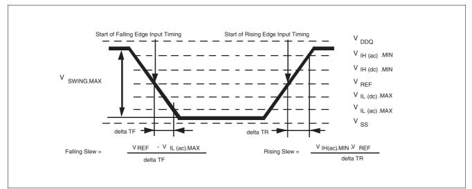
3) AC timings are referenced with input waveforms switching from  $V_{\rm IL(ac)}$  to  $V_{\rm IH(ac)}$  on the positive transitions and  $V_{\rm IH(ac)}$  to  $V_{\rm IL(ac)}$ on the negative transitions.
