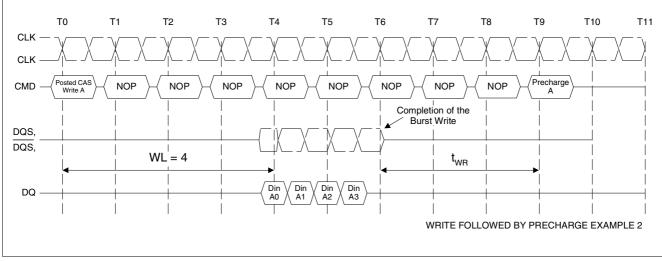
Figure 40 Write followed by Precharge Example 2: WL = (RL - 1) = 4, BL = 4,  $t_{WR}$  = 3
