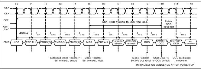
Figure 4 Initialization Sequence after Power Up
