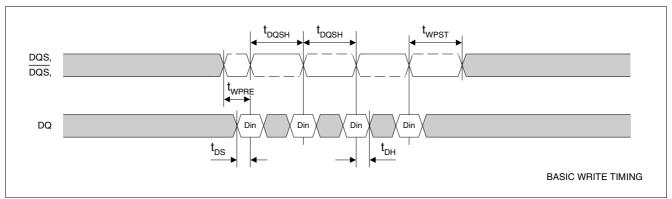
Figure 25 Basic Write Timing
