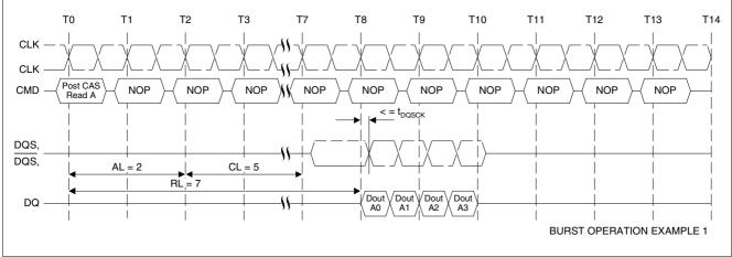
Figure 20 Read Operation Example 1: RL = 7 (AL = 2, CL = 5, BL = 4)
