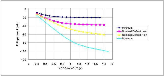
Figure 59 Full Strength Default Pull-up Driver Diagram
