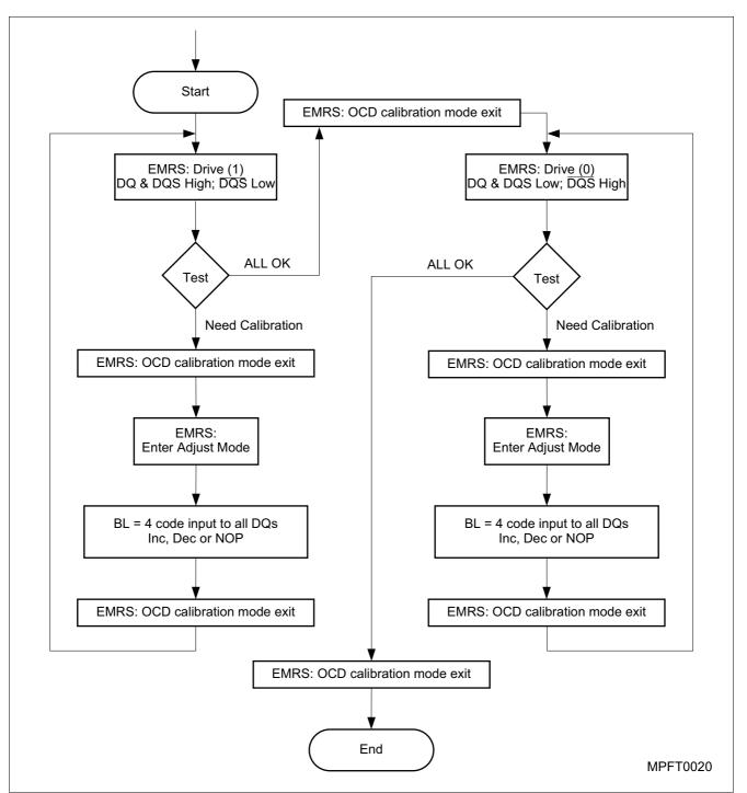
Figure 5 OCD Impedance Adjustment Flow Chart
