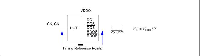
Figure 63 Reference Load for Timing Measurements
