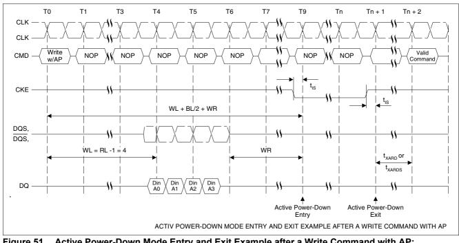
Figure 51 Active Power-Down Mode Entry and Exit Example after a Write Command with AP: WL = 4, WR = 3, BL = 4
