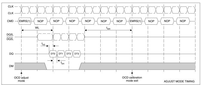
Figure 6 Adjust Mode Timing Diagram
