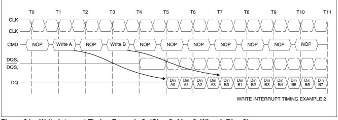
Figure 34 Write Interrupt Timing Example 2: (CL = 5, AL = 0, WL = 4, BL = 8)
