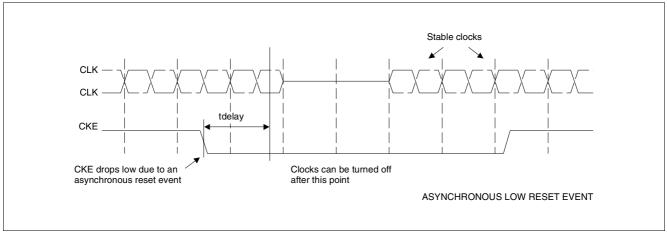
Figure 56 Asynchronous Low Reset Event
