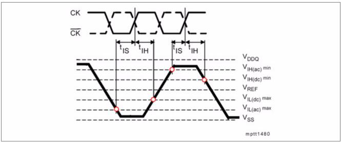
Figure 64 Timing Definition for Input Setup (tIS) and Hold Time (tIH)
