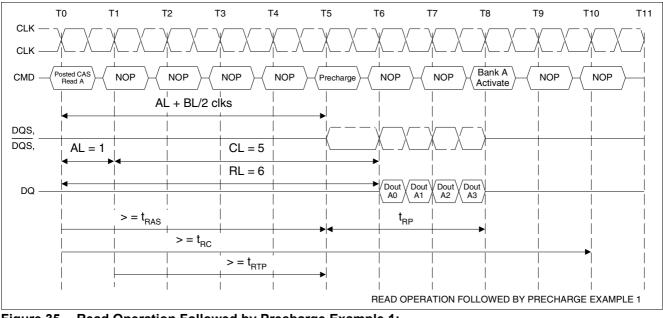
**Read Operation Followed by Precharge Example 1:** Figure 35 RL = 6 (AL = 1, CL = 5), BL = 4,  $t_{RTP} \le 2$  clocks
