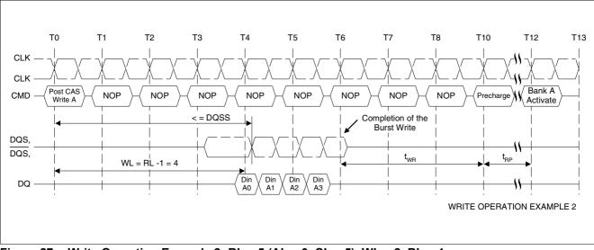
Figure 27 Write Operation Example 2: RL = 5 (AL = 0, CL = 5), WL = 2, BL = 4
