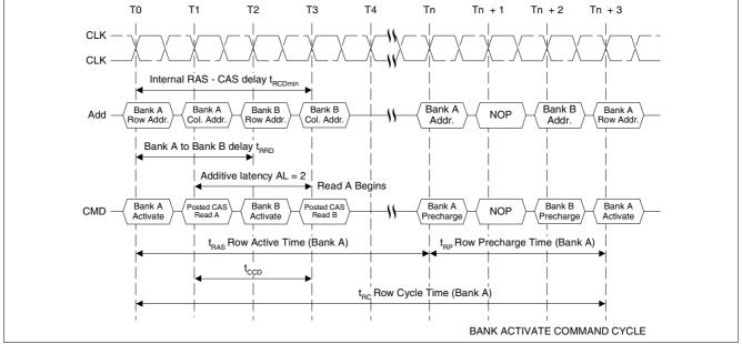
Figure 13 Bank Activate Command Cycle:  $t_{RCD}$  = 3, AL = 2,  $t_{RP}$  = 3,  $t_{RRD}$  = 2
