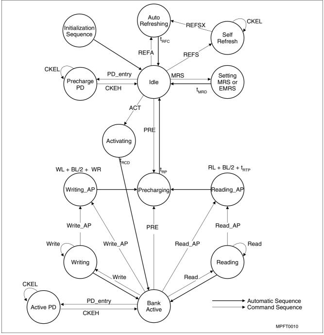
Figure 3 Simplified State Diagram
