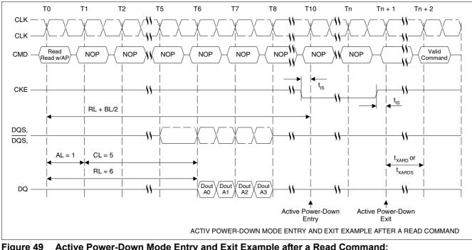
Figure 49 Active Power-Down Mode Entry and Exit Example after a Read Command: RL = 6 (AL = 1, CL =5), BL = 4
