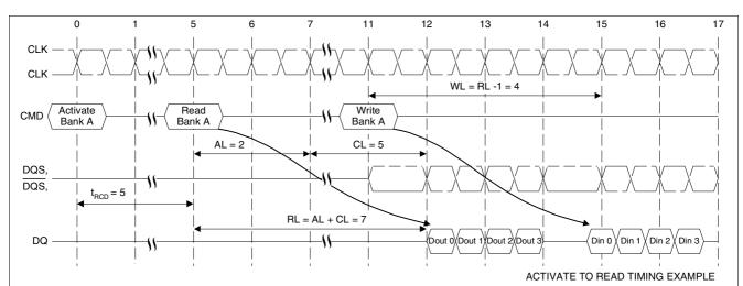
Figure 15 Activate to Read Timing Example: Read followed by a write to the same bank, Activate to Read delay < *t*<sub>RCDmin</sub>: AL = 2 and CL = 5, RL = (AL + CL) = 7, WL = (RL -1) = 6, BL = 4
