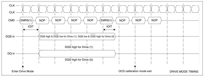
Figure 7 Drive Mode Timing Diagram
