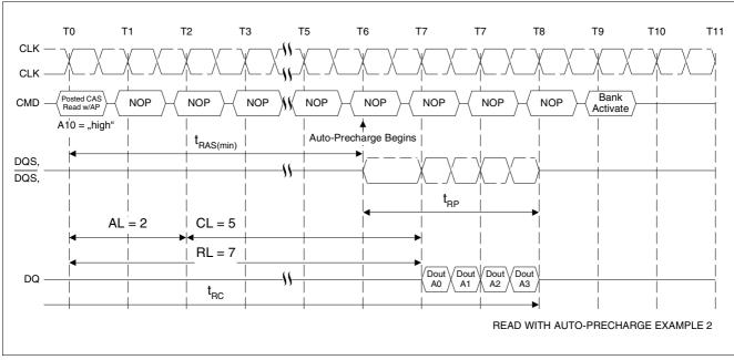
Figure 42 Read with Auto-Precharge Example 2, followed by an Activation to the Same Bank ( $t_{RAS}$  Limit): RL = 7 (AL = 2, CL = 5), BL = 4,  $t_{RTP} \le 2$  clocks
