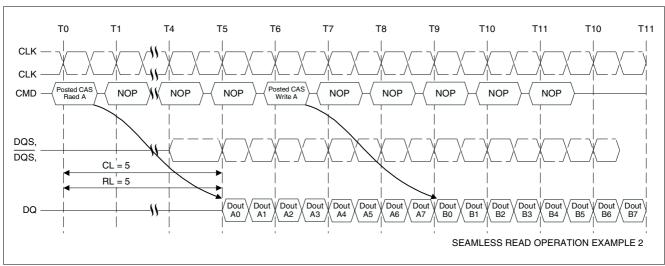
The seamless read operation is supported by enabling a read command at every BL / 2 number of clocks. This operation is allowed regardless of same or different banks as long as the banks are activated.
