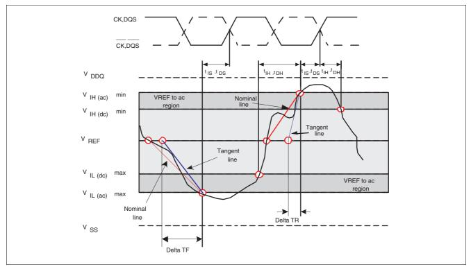
Figure 68 Slew Rate Definition Tangent
