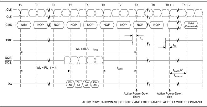
Figure 50 Active Power-Down Mode Entry and Exit Example after a Write Command: WL = 4,  $t_{WTR}$  = 2, BL = 4
