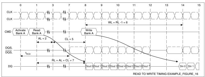
Figure 16 Read to Write Timing Example: Read followed by a write to the same bank, Activate to Read delay  $< t_{\text{RCDmin}}$ : AL = 2 and CL = 5, RL = (AL + CL) = 7, WL = (RL -1) = 6, BL = 8
