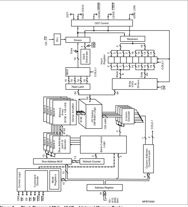
Figure 2 Block Diagram 4 Mbit × 16 I/O × 4 Internal Memory Banks
